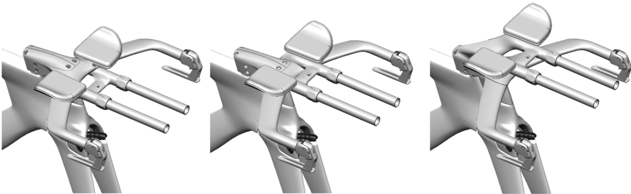
Figure 26 Left to right: X-lo, Low, High-V. The handlebar extensions attach to the arm pad support, which means they go up and down with the arm pads so they are always at the right height for the athlete's hands.
