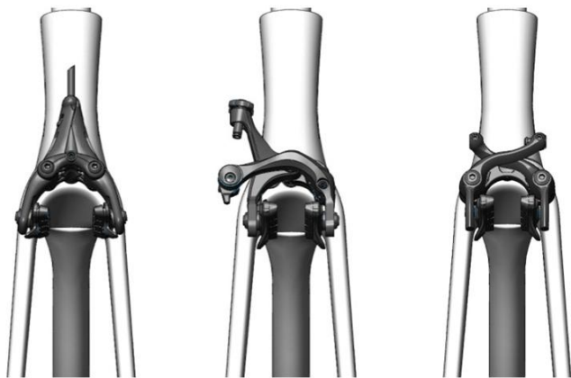
Figure 22 The P5 forks accept any modern road brake that mounts on the traditional center bolt. Left to right: Magura, side pull and center pull.
