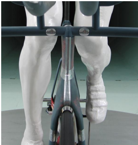
Figure 36 One of a series of SLA models used to measure the sensitivity of aero drag to variations in head tube thickness.
