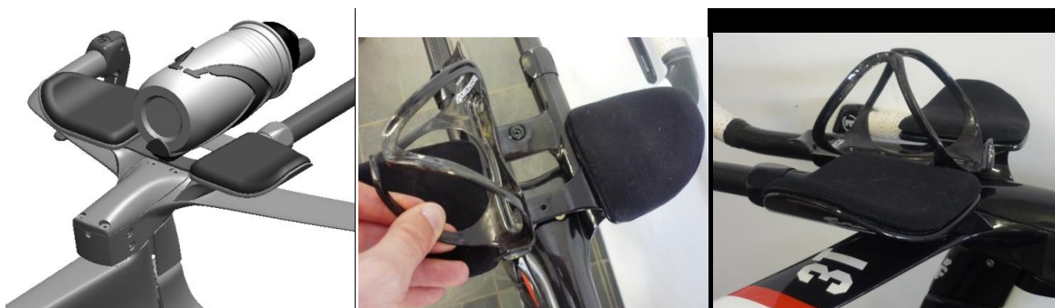
Figure 52 Cervélo P5 aero bar (Low arm pad configuration), showing integrated bottle cage mount.
