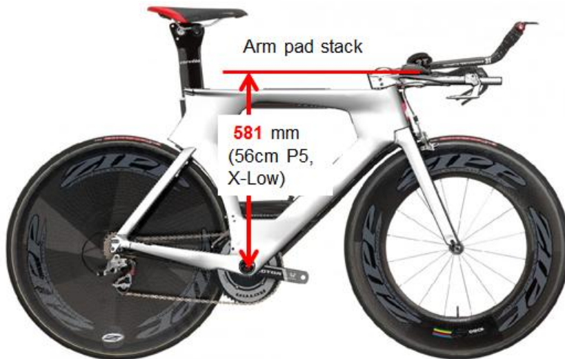
Figure 33 Again the same size 56cm P5, now with the “X-Low” macro height setting. The arm pad stack drops 20mm lower to 581mm.
