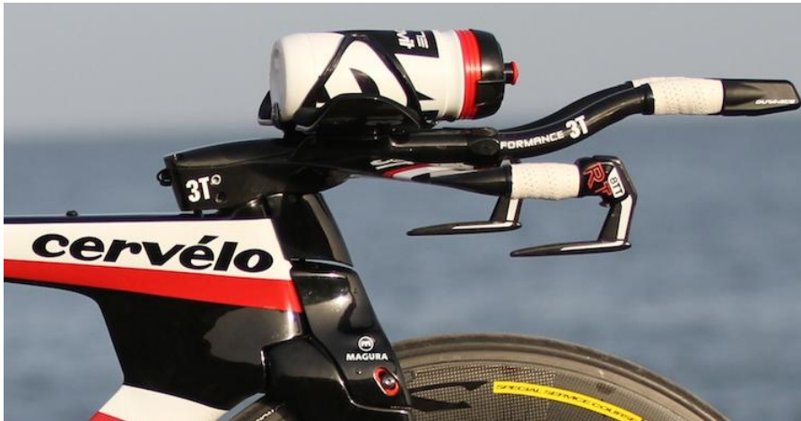
Figure 37 The aero bar's stem is an aero match with the P5 frame and brake.
