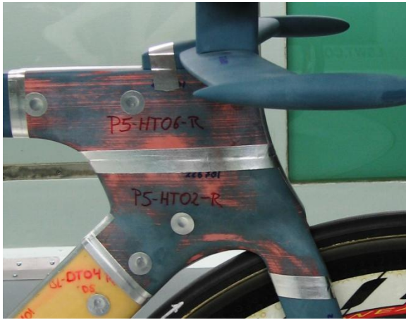
Figure 35 Wind tunnel test prototype for a fully integrated fork, frame, headset, brake and stem concept. It was abandoned in favor of the final P5 concept.
