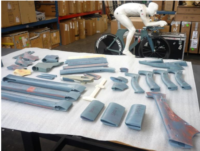
Figure 2 Some of the many prototype skin surfaces designed following the aero zone principle. They are shown here in Cervélo’s R&D lab in Toronto before being packed up in preparation for a trip to the wind tunnel.
