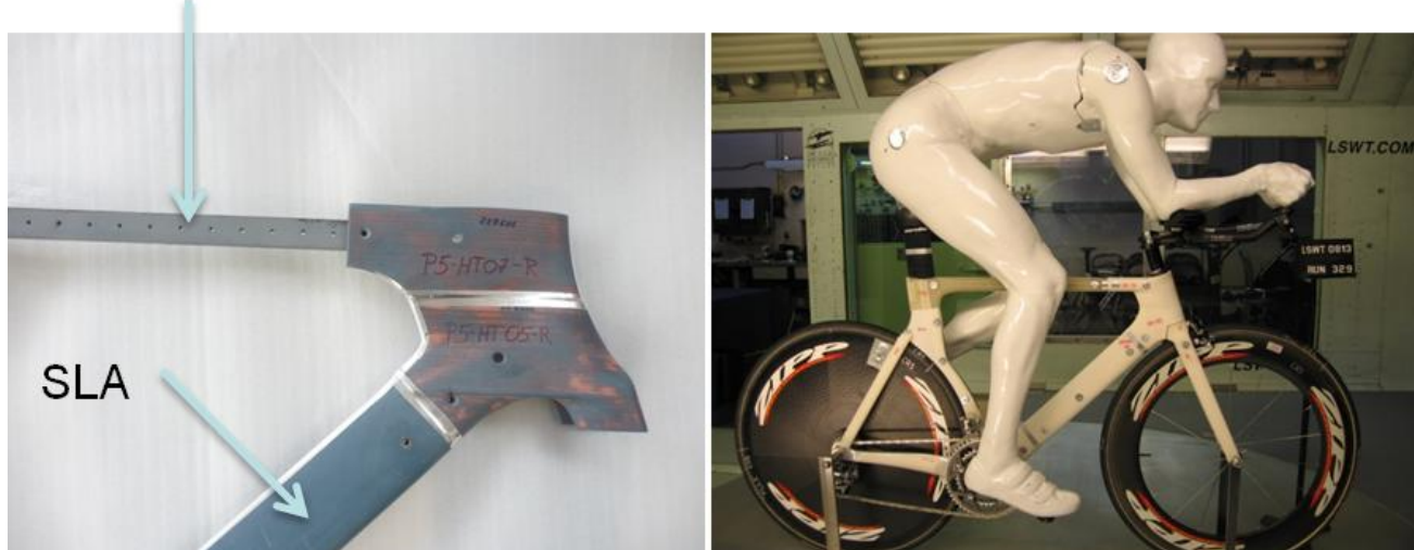
Figure 1 The "test mule" (left) with quick-change SLA (stereo lithography, a rapid prototyping technique) skins. DZ, "foam Dave" aboard the mule in the wind tunnel (right).
