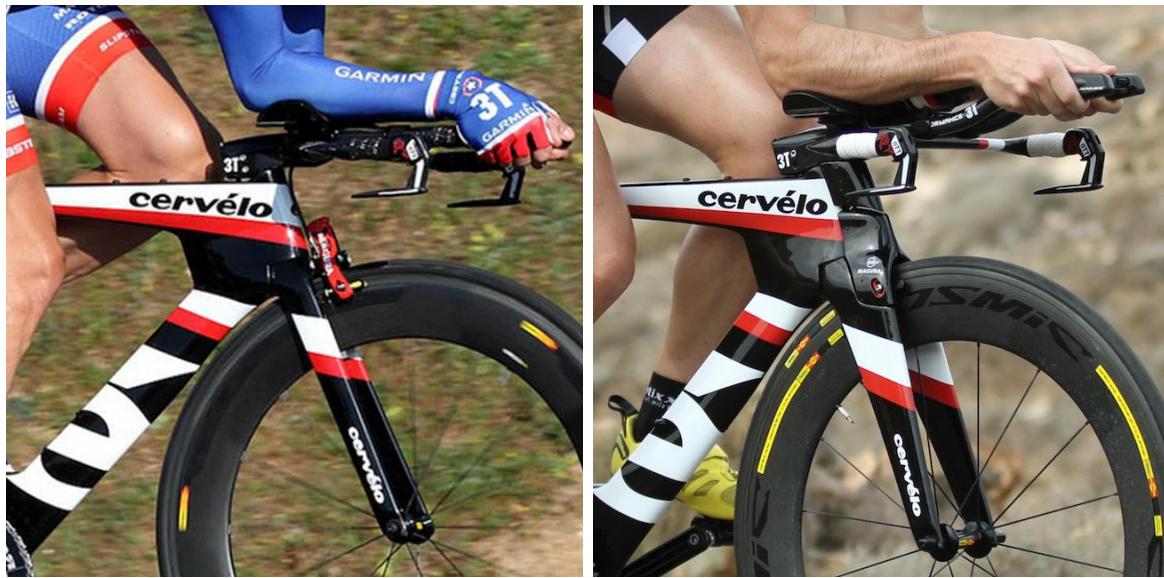
Figure 18 Left: the Cervélo P5-Three fork, 3:1 blades and UCI legal. Right: The Cervélo P5-Six fork, 6:1 blades and UCI-illegal.
