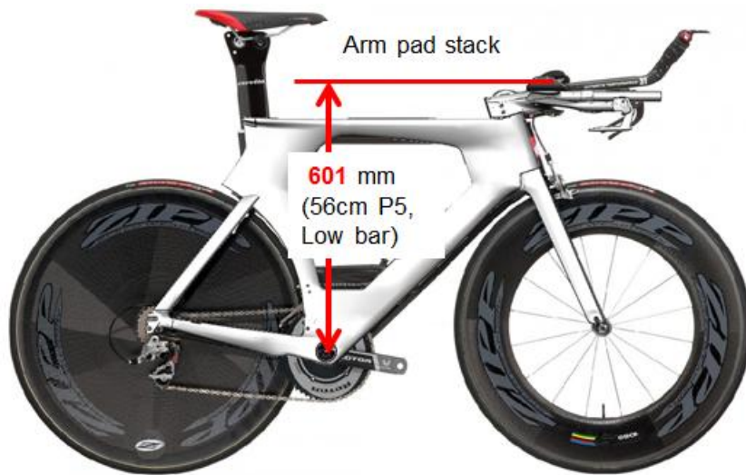
Figure 32 The same size 56cm P5 with “Low” macro height setting has essentially the same arm pad stack at 601mm.
