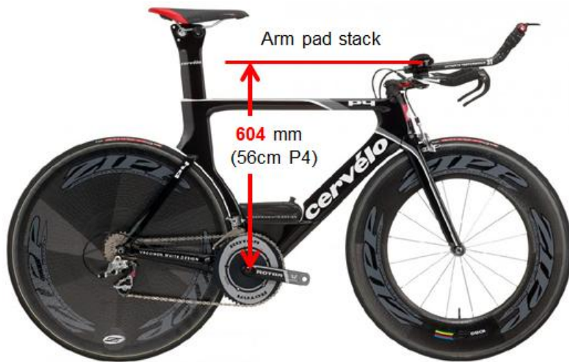
Figure 31 A typically equipped 56cm P4 with low position has an arm pad stack dimension of 604mm.
