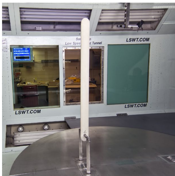
Figure 7: Straight airfoil section (left) and corresponding wheel (right) being tested at the San Diego Low Speed Wind Tunnel.
