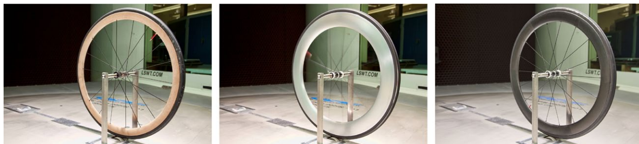
Figure 10: Prototype MDF (left) and aluminum (center) along with a carbon wheel (right) in the San Diego Low Speed Wind Tunnel.
