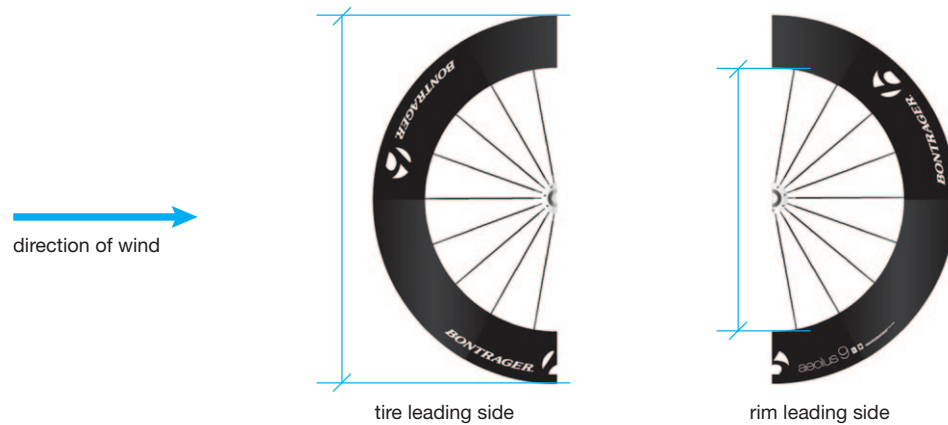
Figure 5: Depiction of the tire-leading and rim-leading sides of a wheel.
