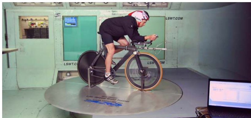
Figure 7: Sensor calibration in the San Diego Low Speed Wind Tunnel.
