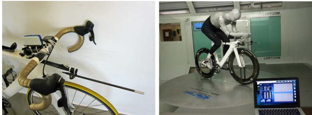
Figure 16: Trek's early production Aerostick sensor (Left) on a Madone and (Right) on a Speed Concept with mannequin during calibration at the San Diego Low Speed Wind Tunnel.
