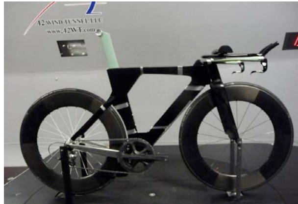
Figure 18: A2 Wind Tunnel, frame skeleton with skins.
