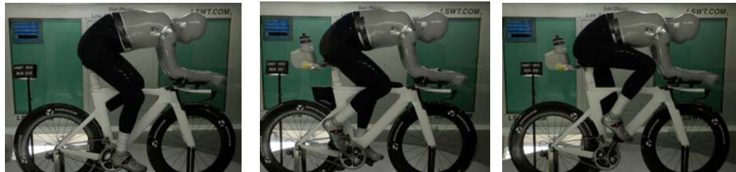
Figure 23: Various storage testing at the San Diego Low Speed Wind Tunnel. (A) New Speed Concept with Manny. (B) New Speed Concept with Manny, Draft Box, Speed Box, and 2-Pack. (C) New Speed Concept with Manny and 2-Pack.
