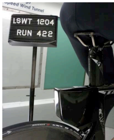
Figure 29: Wider Draft Box. San Diego Low Speed Wind Tunnel, January 2012.
