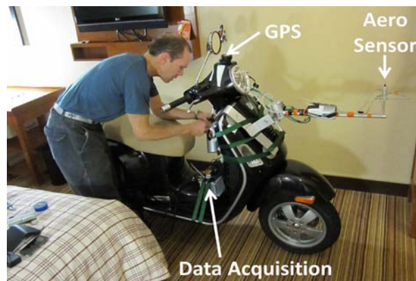
Figure 9: Setting up the scooter in the hotel room before a test.
