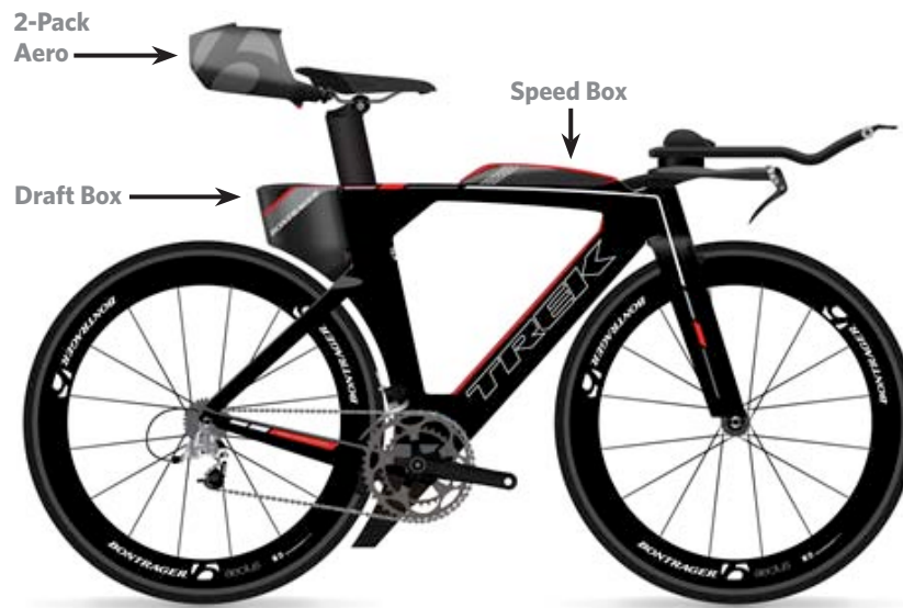
Figure 28: New Speed Concept with Draft Box, 2-Pack, and Speed Box storage.
