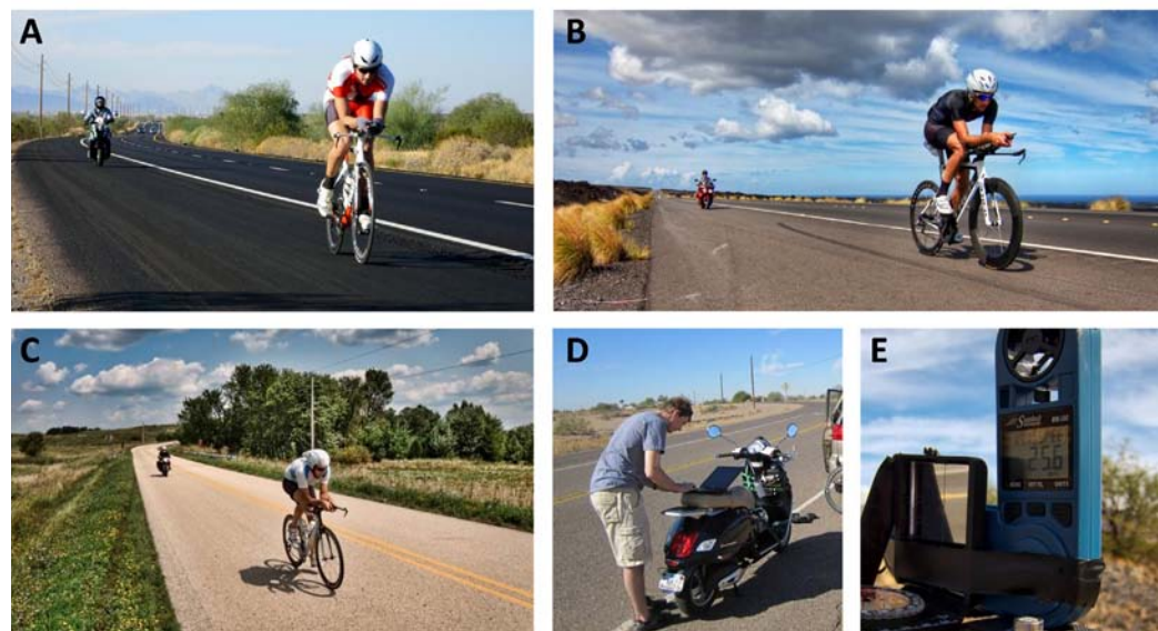
Figure 10: Testing at (A) Arizona Ironman course, (B) Hawaii Ironman course, and (C) Wisconsin Ironman course. (D) Downloading data after a lap in Arizona. (E) Roadside anemometer measurement of a gust in Hawaii.
