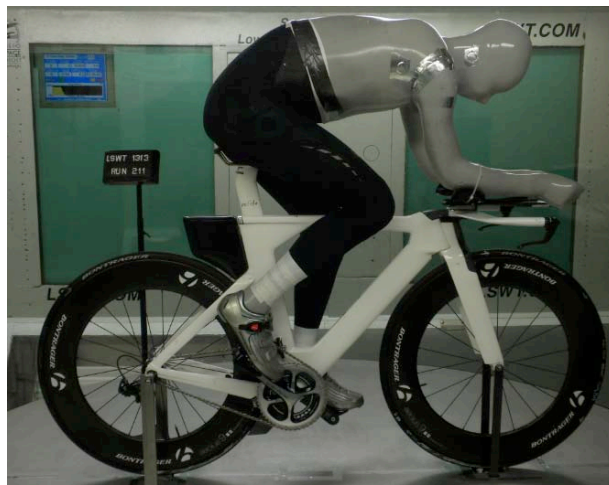
Figure 17: Manny on the new Speed Concept in the San Diego Low Speed Wind Tunnel.
